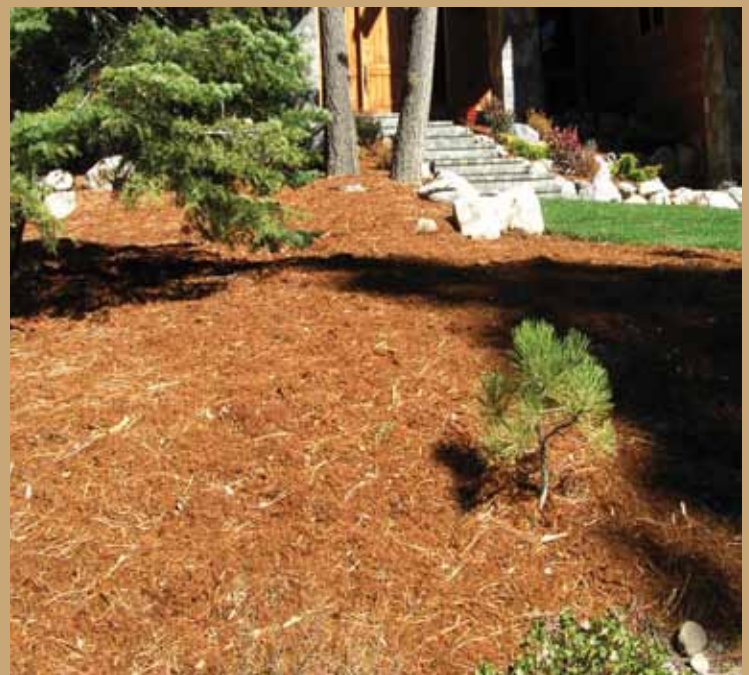
▼ Figure 5. Shredded western red cedar bark, as shown in this photograph, ignited easily and produced the fastest rate of spread of the eight mulch treatments evaluated.
